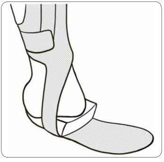
Wedge anterior aspect of calcaneous to previous measurement. If LLD is not fully resolved, it will be necessary to post the heel section of the socket. See page 8, step 5 for illustration.
